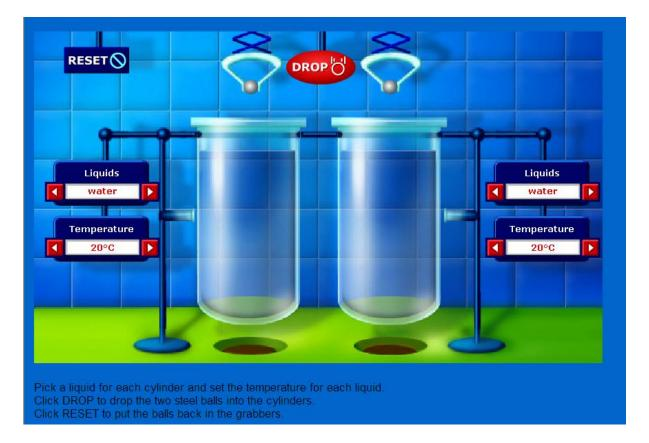
The experiment consists in dropping a ball through different liquids (water, oil, honey...) then observing its speed; it is possible to change liquid temperature by heating with a flame or cooling. Two simultaneous droppings are carried out, after choosing the liquid and the temperature, thus comparing viscosities as function of temperature and substance.
